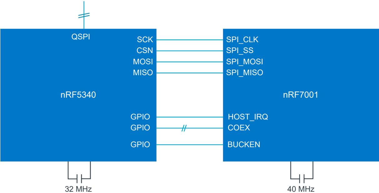
Figure 22: SPI connection
