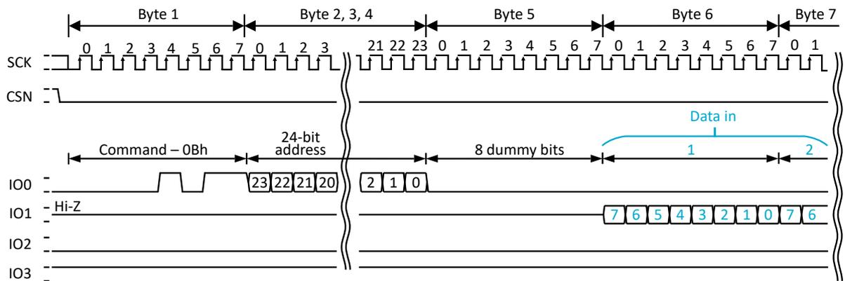
Figure 8: FASTREAD (Read bytes at higher speed)
