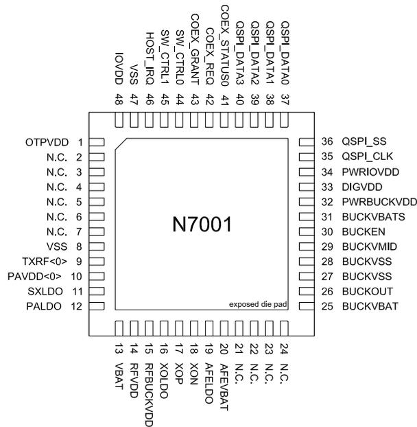
Figure 17: Pin assignments
