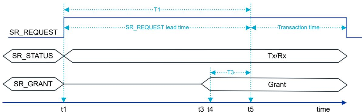
Figure 15: 3-wire timing without priority multiplexing
