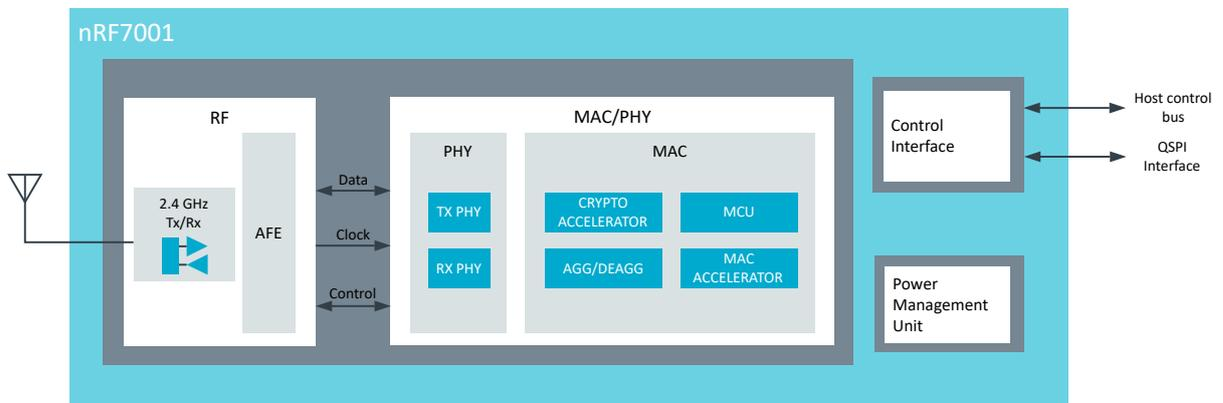
Figure 1: nRF7001 block diagram
