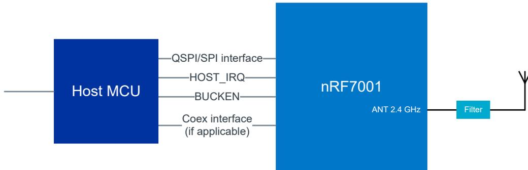
Figure 2: Functional block diagram with generic host *MCU*
