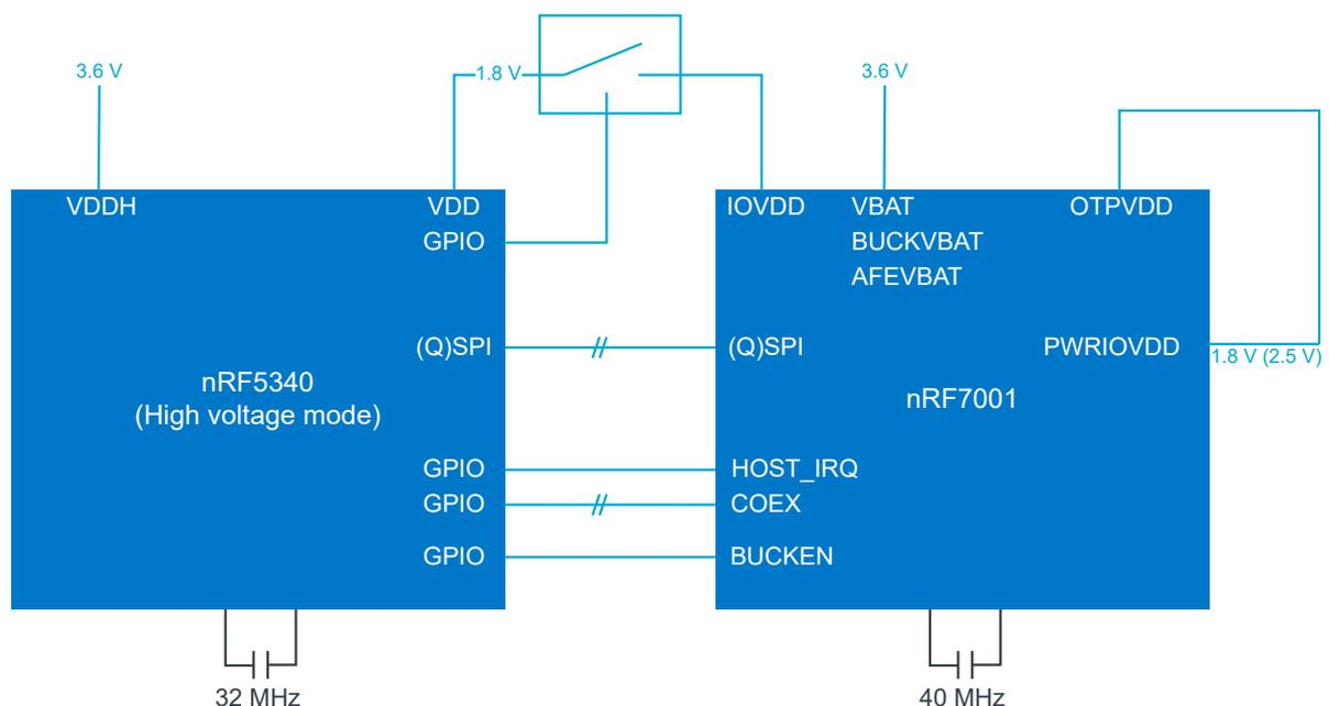
Figure 19: Supply system - high voltage mode
