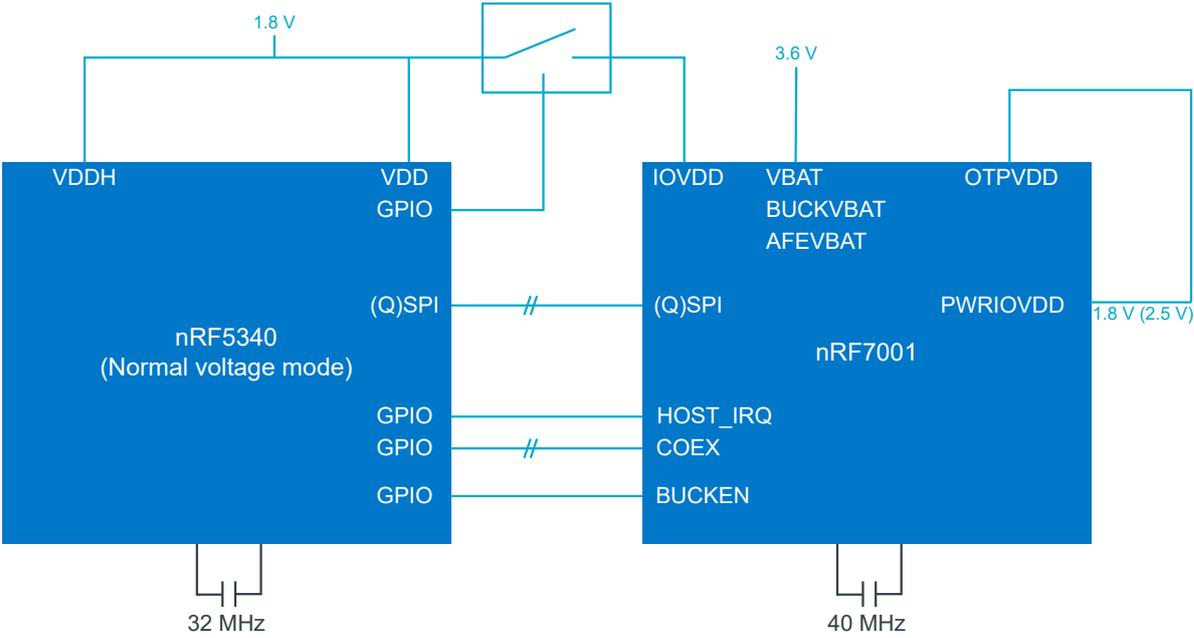
Figure 20: Supply system - normal voltage mode
